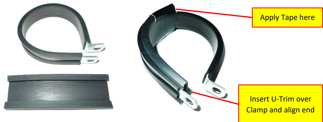
Figure 11 – Rubber U-Trim over Loop Clamp
