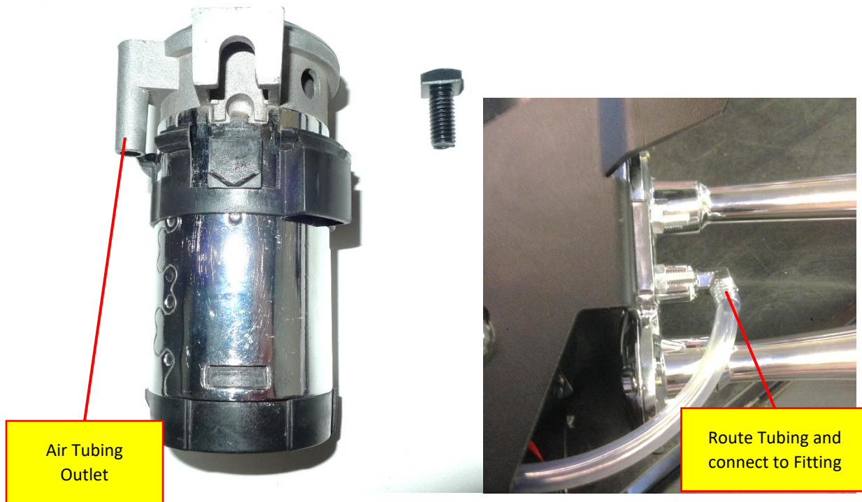
Figure 15 – Air Compressor to Air Horn Tubing (back view shown with Trumpets)
