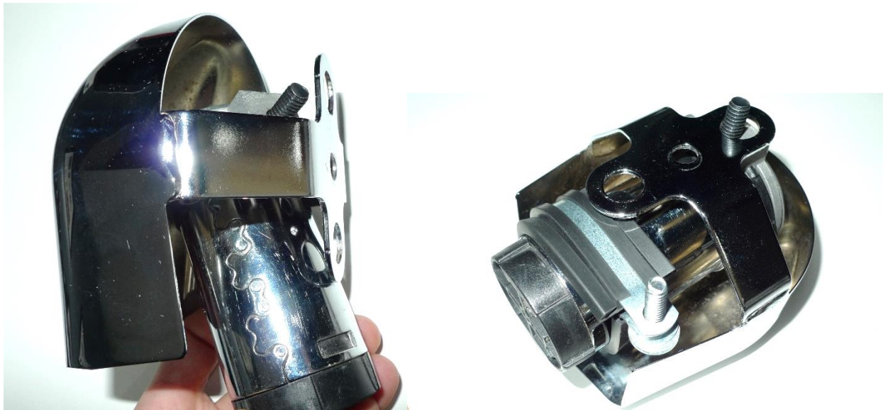
Figure 13 – Air Compressor inserted into Horn Cover
