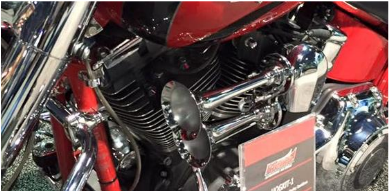
Figure 17 – Air Horn assembly installed
